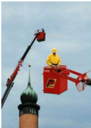
Work platform assembled with a variable reach lift truck
